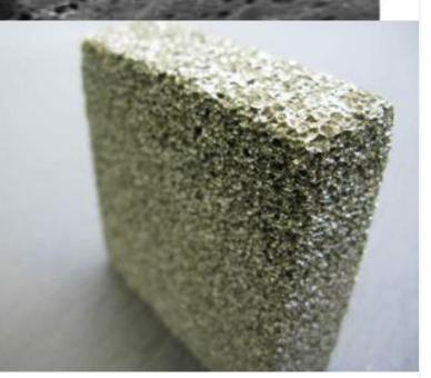
Aim: synthesis of commercially comparable Foam glass (*FG*) material from powder mixture of sewage sludge ash (SSA), recycled bottle glass culet (G), and carbonate foaming agent (F), determination of *FG* environmental impact
